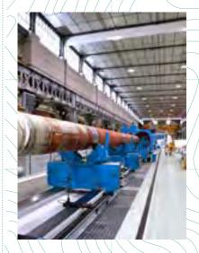
NAVAL GROUP IS INVESTING HEAVILY TO UPGRADE ITS INDUSTRIAL TOOL. AT ANGOULÊME-RUELLE, TWO NEW INDUSTRIAL MACHINING FACILITIES HAVE BEEN SET UP TO OPTIMISE THE MACHINING AND DRILLING CAPACITIES FOR THE SHAFT LINES, STRATEGIC COMPONENTS FOR THE SHIPS' PROPULSION
